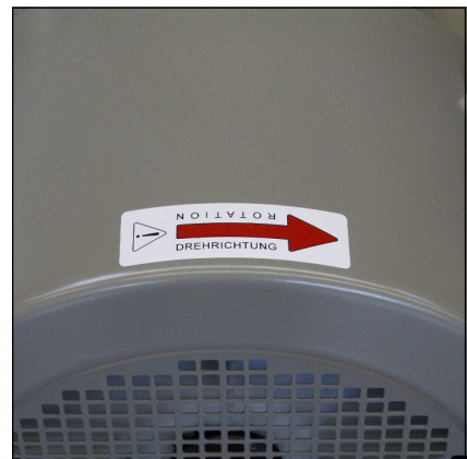
Fig. 1 - Rotary direction arrow (motor)
