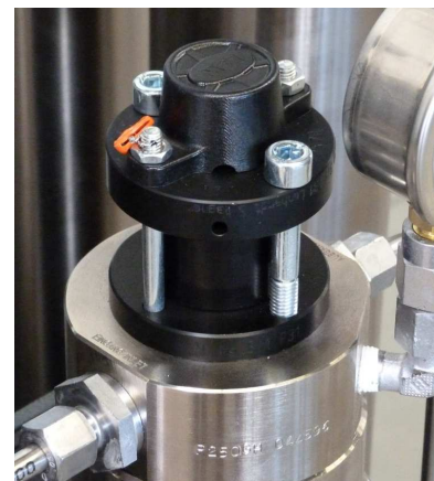
Safety valve 4th stage
