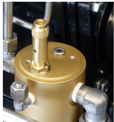
Safety valve 3rd stage
