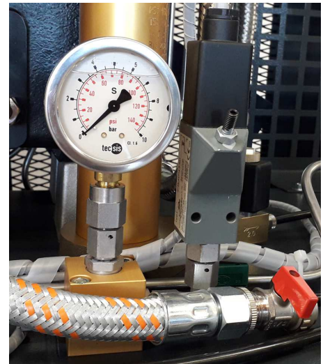
Oil pressure switch and oil pressure gauge
