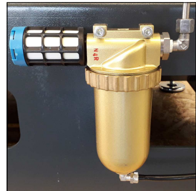
Oil / water separators final stage
