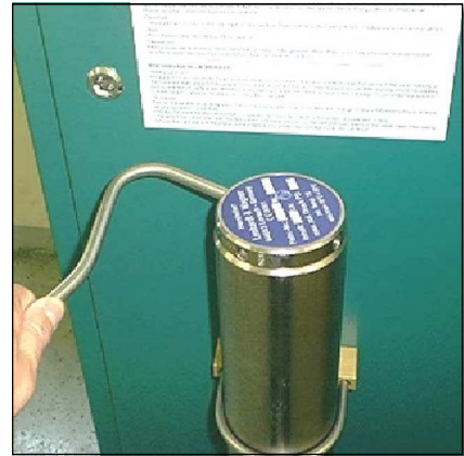
Fig. 1 - Unscrew the filter housing cover.
