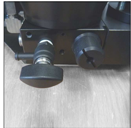
Fig. - Pressure maintaining / non return valve in the filter base and HP-outlet
