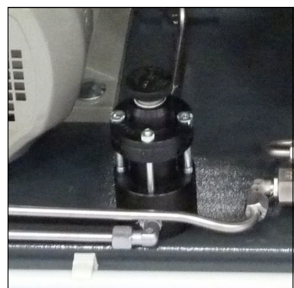
Safety valve 3rd stage
