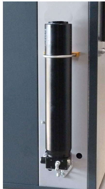
Oil / water separators final stage
