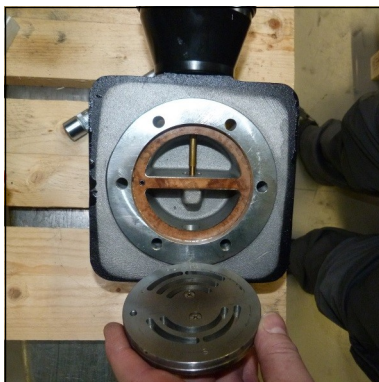
Fig. 2 - Correct position of in and outlet valve
