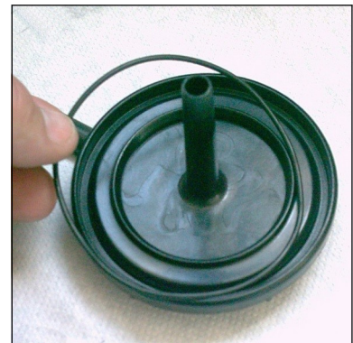
Fig. 3 - Place o-ring into the filter housing
