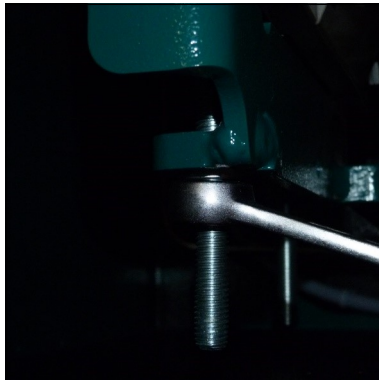
Fig. 2 - Tighten V-belt by the lock nut
