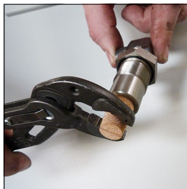
Fig. 3 - Change sinter filter
