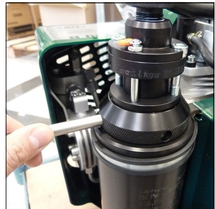
Fig. 1 - Loosen filter housing topcap by using the filter tool
