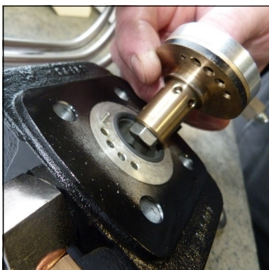
Fig. 1 - Ensure correct valve position (centre pin)
