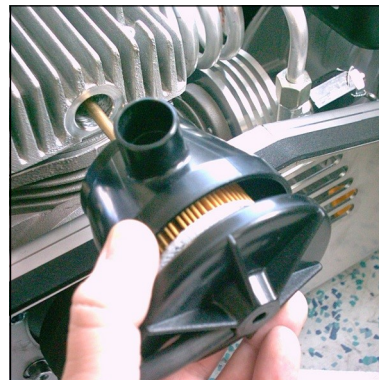
Fig. 2 - Pull out filter housing carefully
