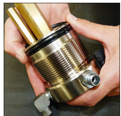
Fig. 4 - Change o-ring and back-up rings
