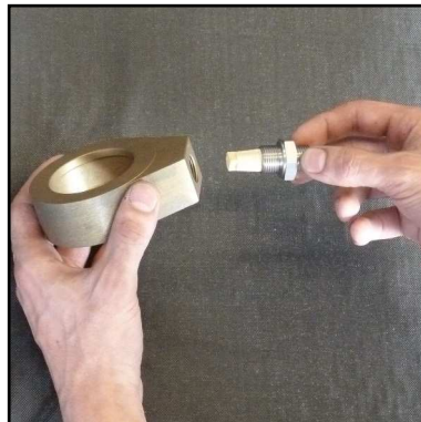
Abb. 8 - Change sinter filter
