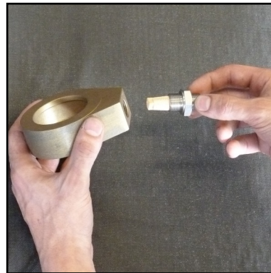
Abb. 8 - Change sinter filter
