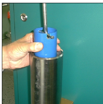
Fig. 4 - Pull the cartridge out of the housing.
