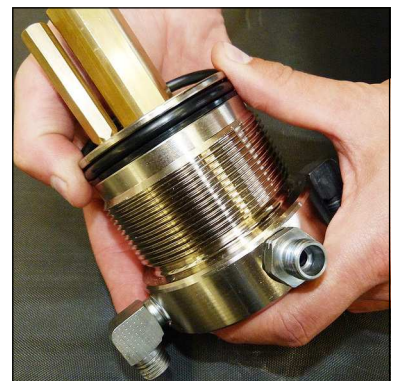
Fig. 4 - Change o-ring and back-up rings
