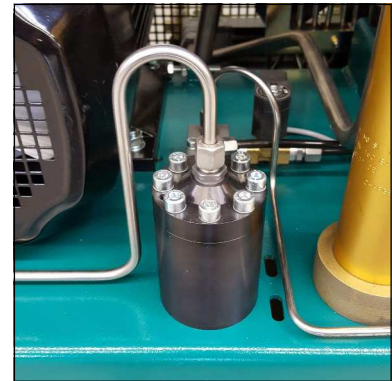
Fig. 1 - Condensate stop valve housing
