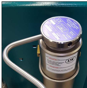
Fig. 2 - Unscrew the filter housing cover.
