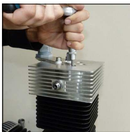
Fig. 1 - Loose valve head screws
