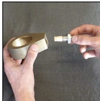
Abb. 8 - Change sinter filter
