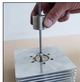
Fig. 3 - Remove in- / outlet valve
