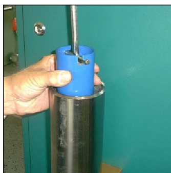
Fig. 4 - Pull the cartridge out of the housing.
