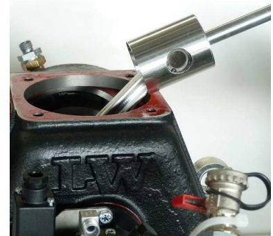
Fig. 2 - Piston 3rd Stage
