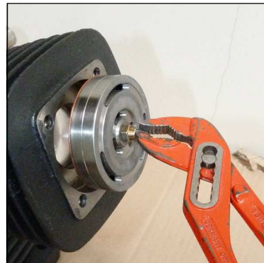
Fig. 2 - Pull out inlet and outlet valve
