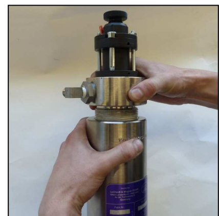
Fig. 3 - Open pre-filter cover
