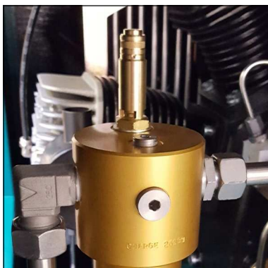
Safety valve 1st stage
