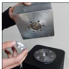
Fig. 2 - Remove lower valve gasket
