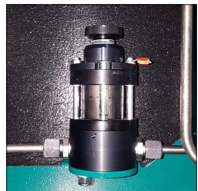
Safety valve 4th stage
