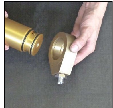
Abb. 6 - Remove the base ring
