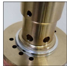
Fig. 4 - Ensure correct mounting position of the upper valve gasket
