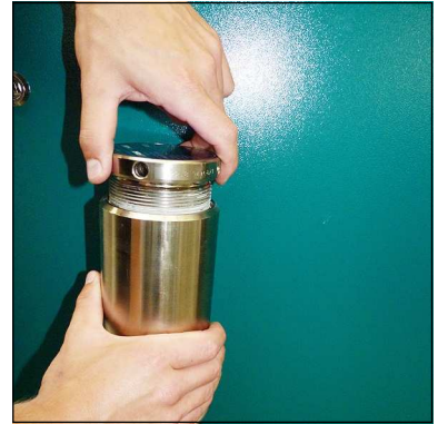
Fig. 1 - Open Filter cover
