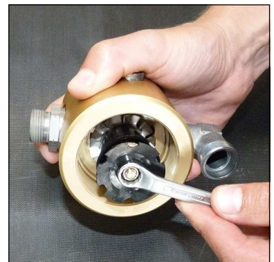
Fig. 2 - Loosen nut at the separator top
