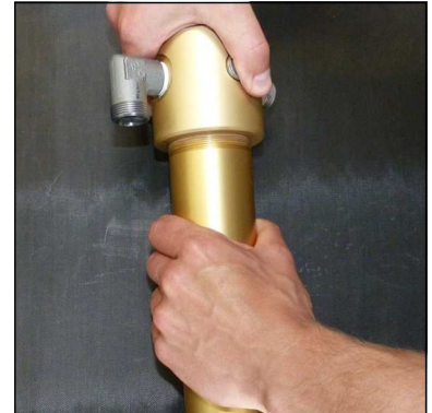
Fig. 1 - Unscrew and remove filter top
