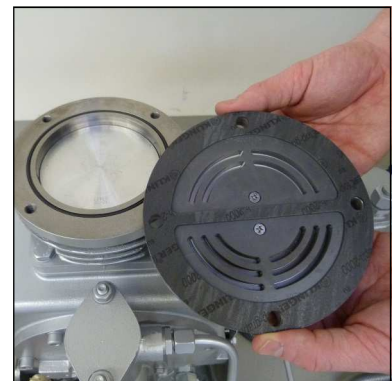
Fig. 2 - Correct mounting position of upper valve gasket
