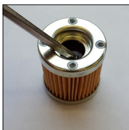
View bypass valve
