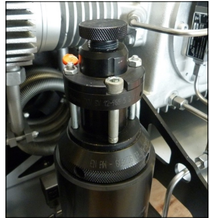
Fig. - Safety valve 3rd stage
