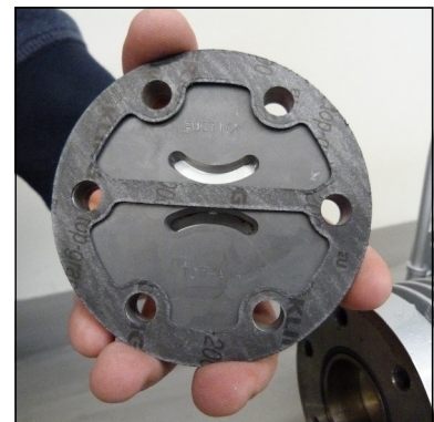
Fig. 2 - Correct mounting position of upper valve gasket
