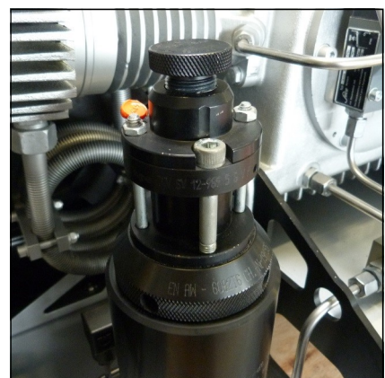
Fig. - Safety valve 3rd stage
