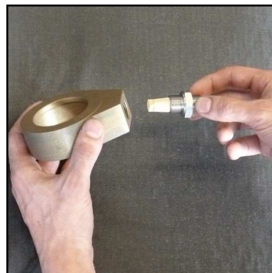
Abb. 8 - Change sinter filter
