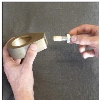
Abb. 8 - Change sinter filter
