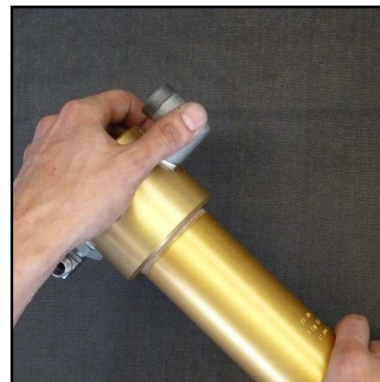
Fig. 1 - Unscrew and remove filter top
