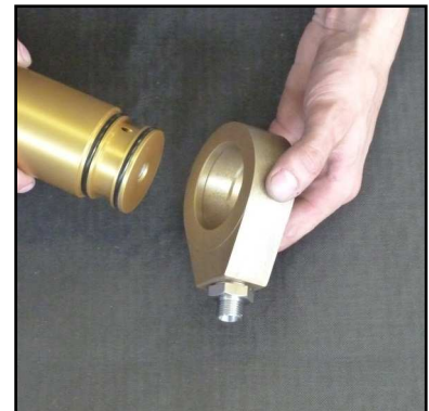
Abb. 6 - Remove the base ring
