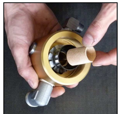
Fig. 3 - Change sinter filter
