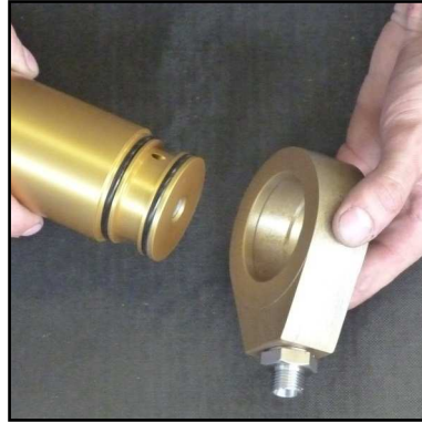
Abb. 5 - Remove the base ring
