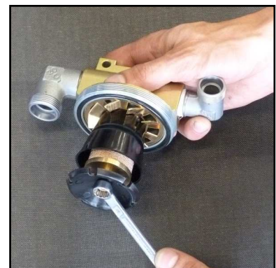
Fig. 2 - Loosen nut at the separator top
