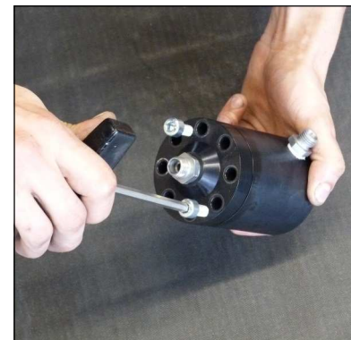
Fig. 2 - Remove the cover
