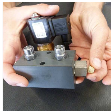
Fig. 3 - Change sinter filter
