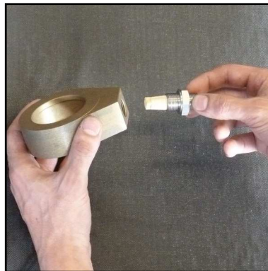
Abb. 8 - Change sinter filter
