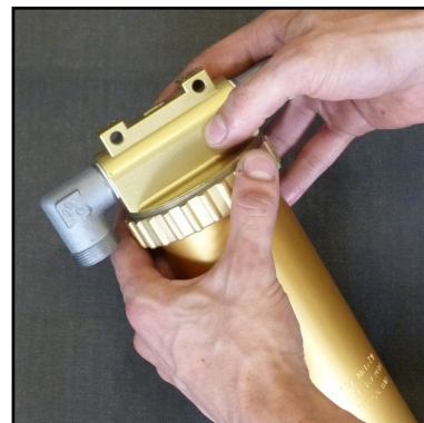
Fig. 1 - Open ring nut and remove separator top
