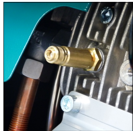
Safety valve 1st stage
