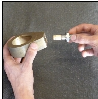
Abb. 8 - Change sinter filter
