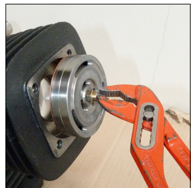
Fig. 2 - Pull out inlet and outlet valve
