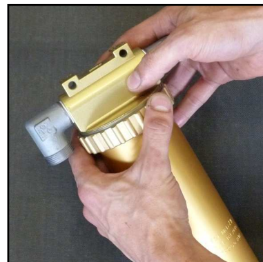
Fig. 1 - Open ring nut and remove separator top
