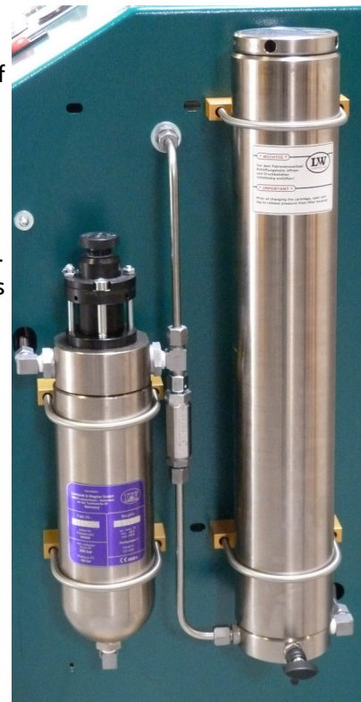
Filterhousing 1.7l (right), and filter unit 0,8l with safety valve (left)
