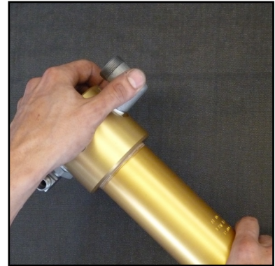
Fig. 1 - Unscrew and remove filter top
