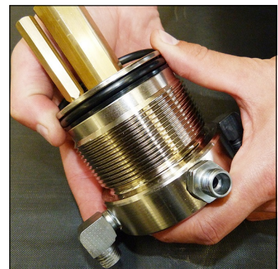
Fig. 4 - Change o-ring and back-up rings
