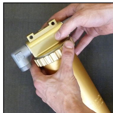
Fig. 1 - Open ring nut and remove separator top
