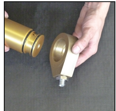
Abb. 6 - Remove the base ring
