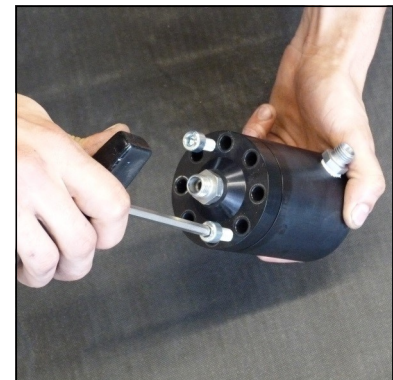
Fig. 2 - Remove the cover
