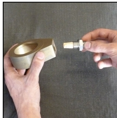
Abb. 8 - Change sinter filter
