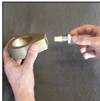
Abb. 8 - Change sinter filter
