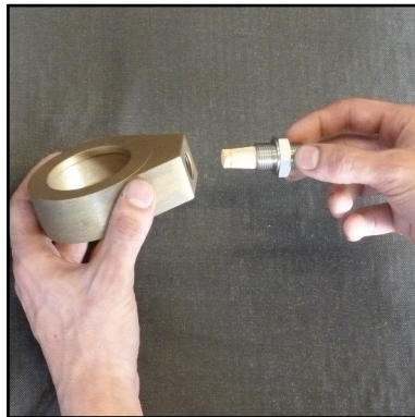
Abb. 7 - Change sinter filter
