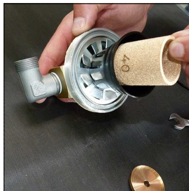
Fig. 3 - Change sinter filter
