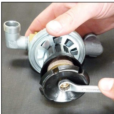
Fig. 2 - Loosen nut at the separator top
