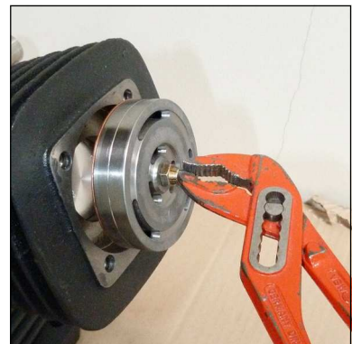
Fig. 2 - Pull out inlet and outlet valve
