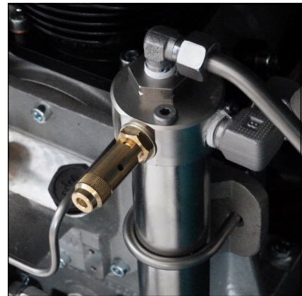
Safety valve 1st stage
