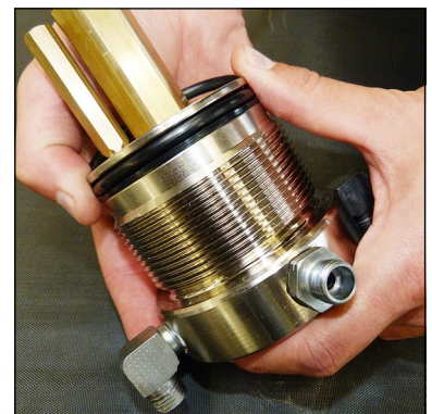
Fig. 4 - Change o-ring and back-up rings
