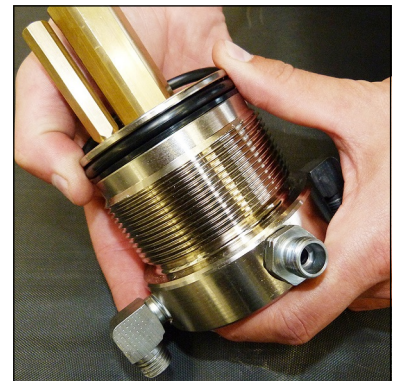
Fig. 4 - Change o-ring and back-up rings
