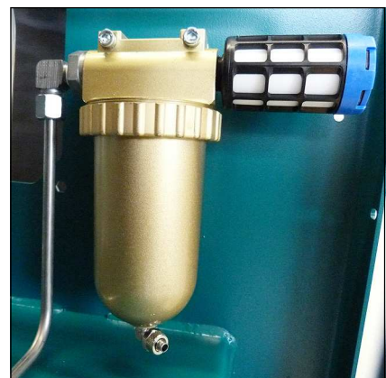
Oil / water separators final stage
