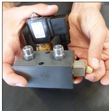
Fig. 3 - Change sinter filter
