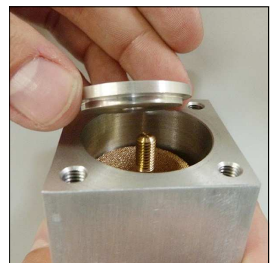
Fig. 5 - Place filter washer and washer
