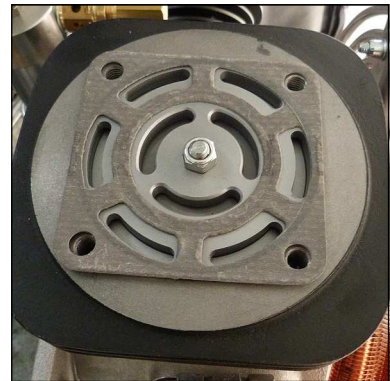
Fig. 4 - Place and align upper valve gasket
