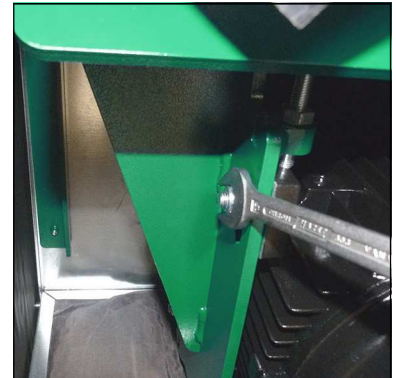
Fig. 1 - Loosen mounting screws
