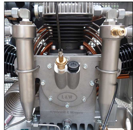
Oil / water separators 1st and 2nd stage
