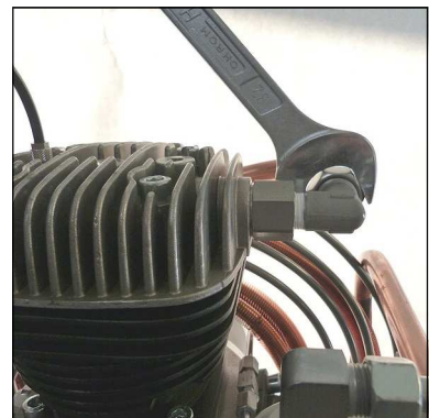
Fig. 6 - Connect pipe connections and tighten
