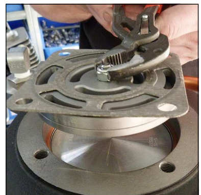
Fig. 2 - Pull out inlet and outlet valve
