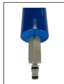
Fig. 5 Installed Filler Adapter
