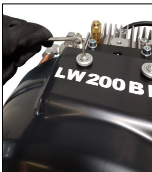
Fig. 1 Loosen Mounting Screws of the Fan Guard
