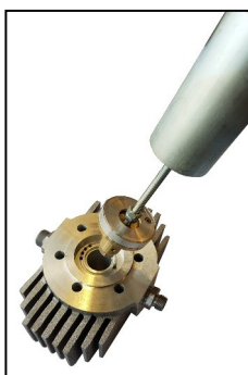
Fig. 4 Remove Inlet / Outlet Valve
