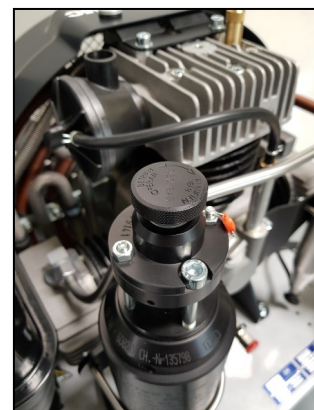
Fig. 3 Safety Valve 3rd Stage
