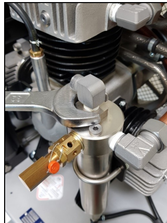
Fig. 2 Loosen Screw Connection
