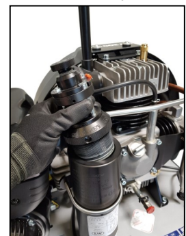
Fig. Remove the Filter Housing Cover
