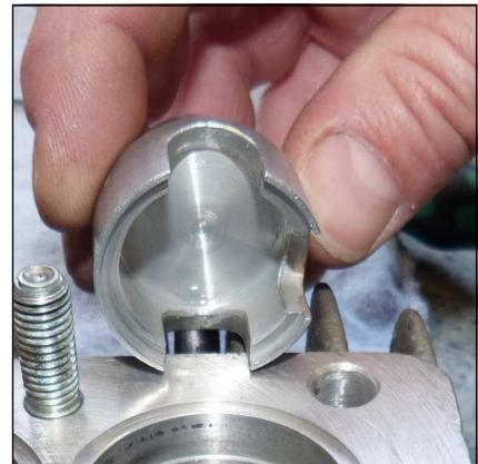
Fig. 1 - Outlet valve holder 1st. stage
