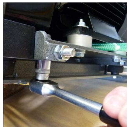
Fig. 1 - Loosen mounting screws of the motor flange
