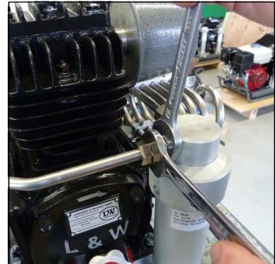
Fig. 1 - Loosen pipe connections of the water separator
