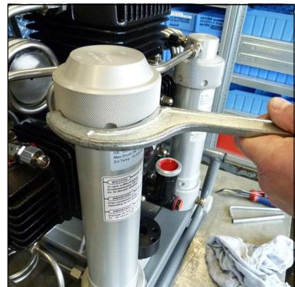
Fig. 1 - Filter housing with filter tool
