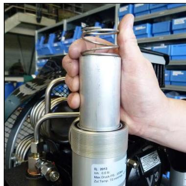
Abb. 2 - Remove filter cartridge
