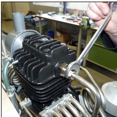
Fig. 2 - Pipe connection
