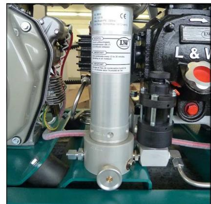
Fig. 2 - Oil- / water separator 3rd stage
