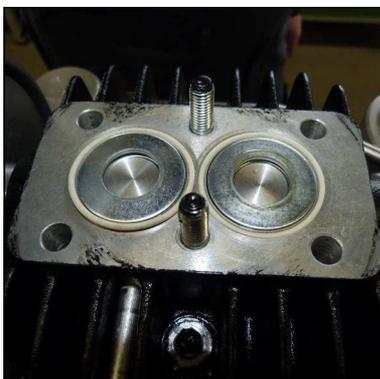
Fig. 5 - Spring plate inside the valve head
