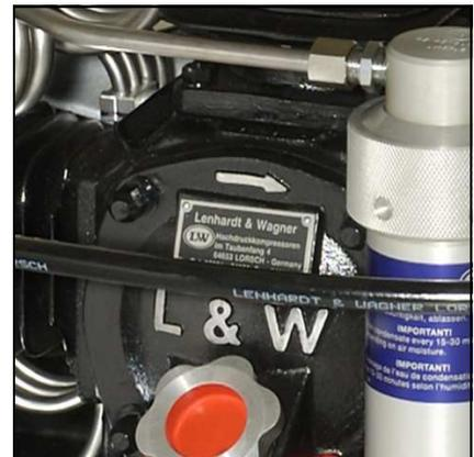
Rotation direction arrow on the compressor block
