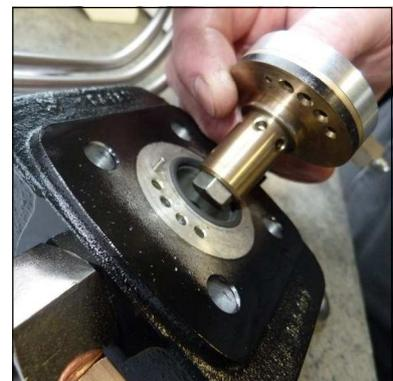
Fig. 4 - Ensure correct valve position (centre pin)
