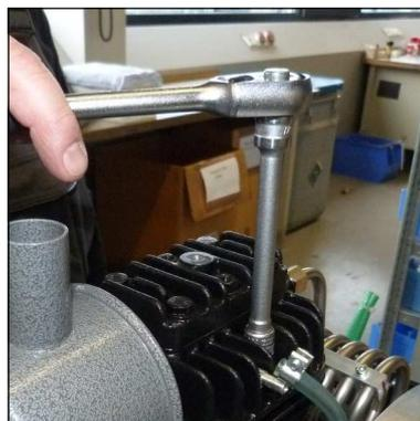
Fig. 6 - Tighten valve head
