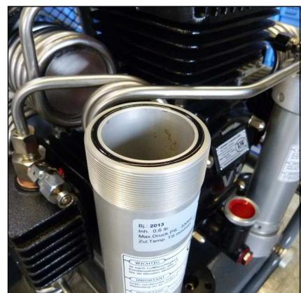
Fig. 2 - Filter housing without filter cover
