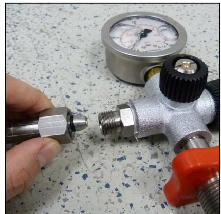
Fig. 2 - O-ring at the filling hose
