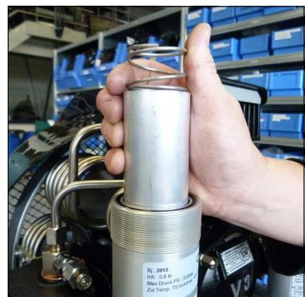
Fig. 3 - Filter cartridge and spring
