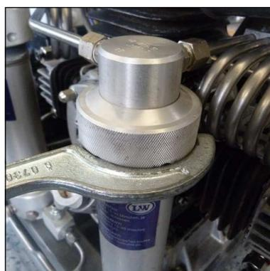
Abb. 5 - Tighten lock ring
