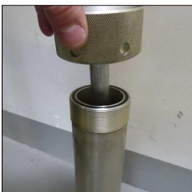
Abb. 4 - Remove lock ring and change o-ring
