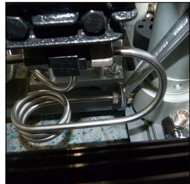
Fig. 2 - Loosen pipe connections of the filter housing
