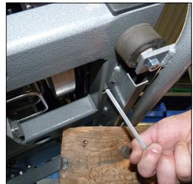
Fig. 3 - Loosen both bottom mounting screws
