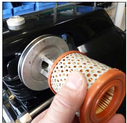
Fig. 3 - Change intake filter
