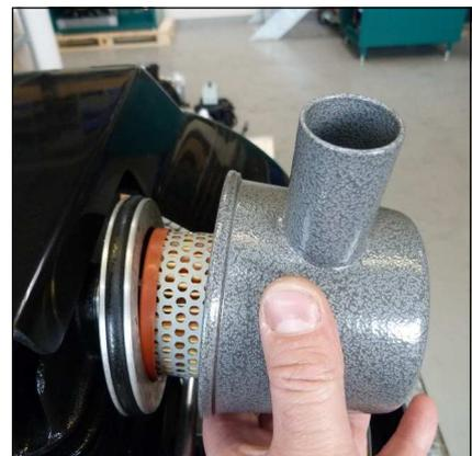
Fig. 2 - Remove intake filter housing cover
