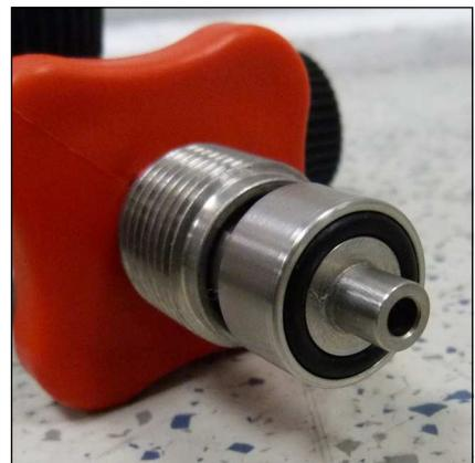
Fig. 1 - O-ring at the filling valve
