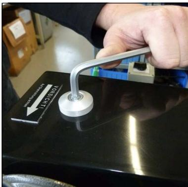
Fig. 1 - Remove top mounting screws
