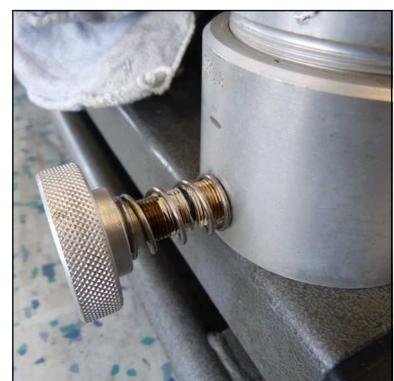
Abb. 6 - O-ring, condensate drain valve
