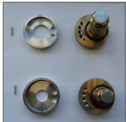
Fig. 2 - In – and outlet valve c/w gaskets
