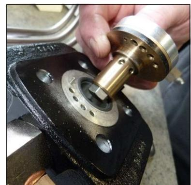
Fig. 5 - Ensure correct valve position (centre pin)
