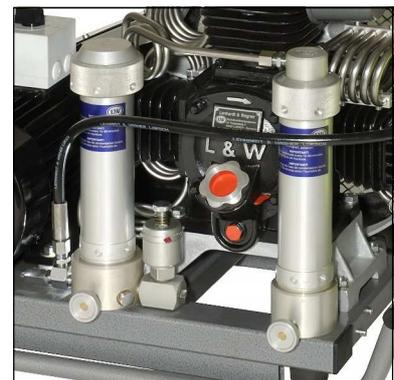
Fig. 1 - Manual condensate drain
