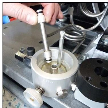
Abb. 5 - Remove duct collar and change o-rings
