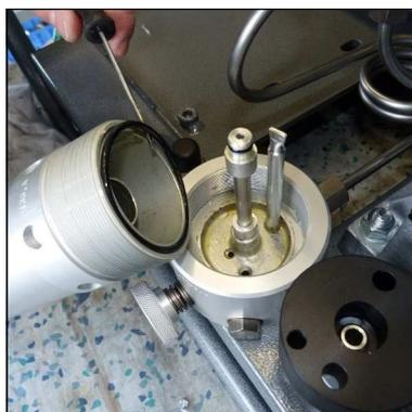
Abb. 4 - Remove lock ring
