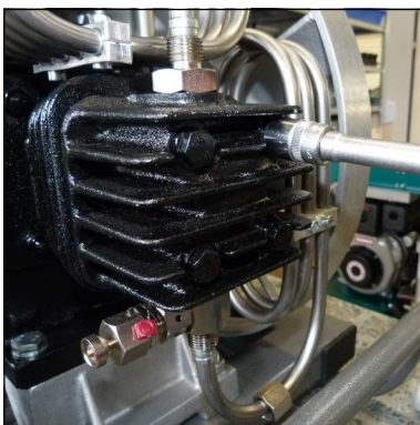
Fig. 2 - Loosen valve head screws
