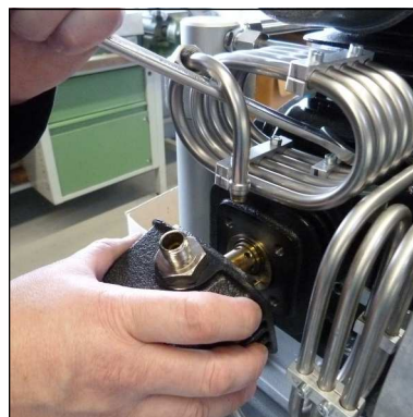
Fig. 3 - Remove valve head
