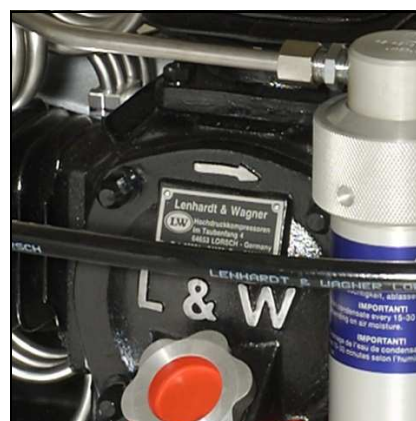
Rotation direction arrow on the compressor block
