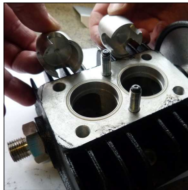
Fig. 3 - Valve bracket positioning
