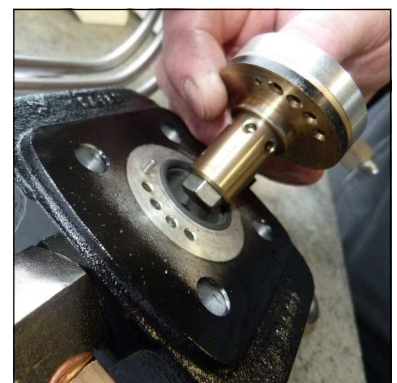
Fig. 5 - Ensure correct valve position (centre pin)
