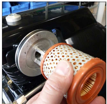
Fig. 3 - Change intake filter
