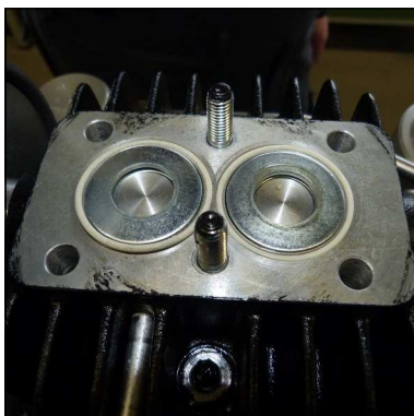
Fig. 5 - Spring plate inside the valve head
