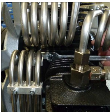
Fig. 3 - Remove mounting screws from the cooling pipe bracket
