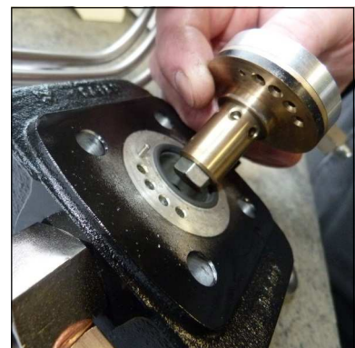
Fig. 4 - Ensure correct valve position (centre pin)
