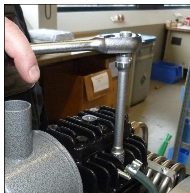
Fig. 6 - Tighten valve head
