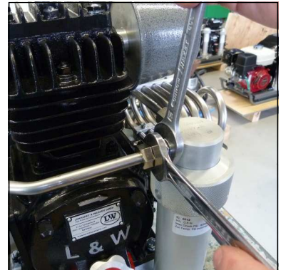
Fig. 1 - Loosen pipe connections of the water separator
