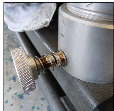
Abb. 6 - O-ring, condensate drain valve
