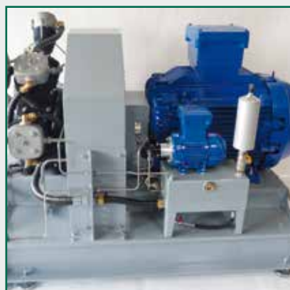
LW1300 EG with additional oil lubrication circuit
