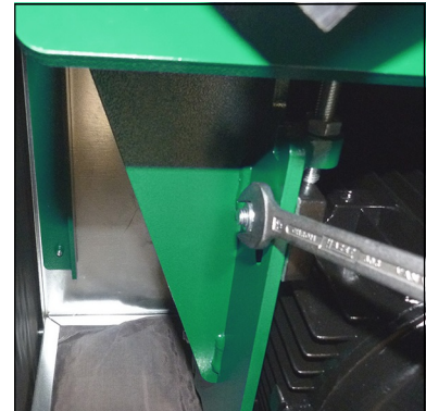
Fig. 1 - Loosen mounting screws
