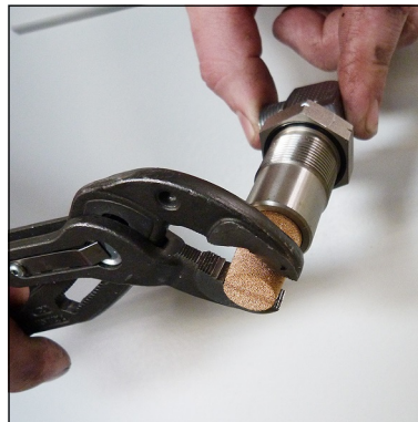
Fig. 3 - Change sinter filter
