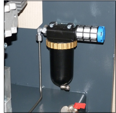
Oil / water separators final stage
