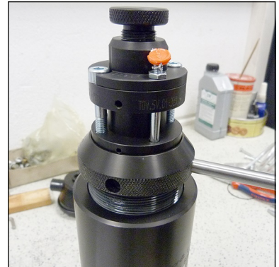
Fig. 1 - Remove/screw in filter cover
