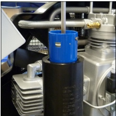
Fig. 2 - Pull out the filter cartridge by the catch and insert a new cartridge
