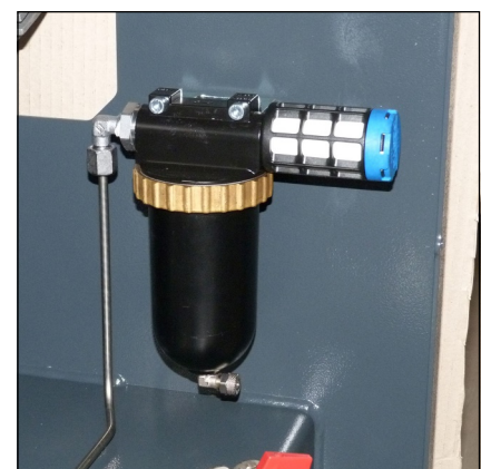
Oil / water separators final stage
