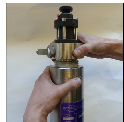
Fig. 3 - Open filter cover
