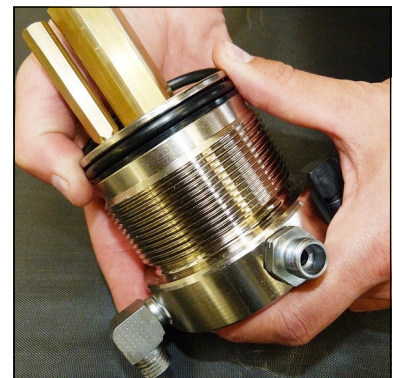
Fig. 4 - Change o-ring and back-up rings
