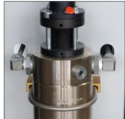
Fig. 1 - Loosen pipe connections and mounting screws
