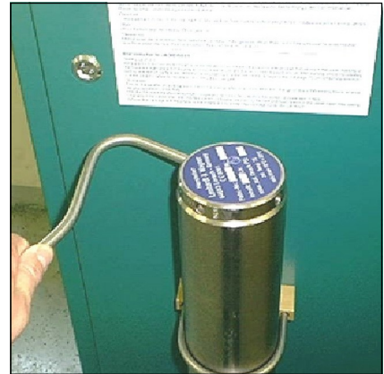
Fig. 1 - Unscrew the filter housing cover.
