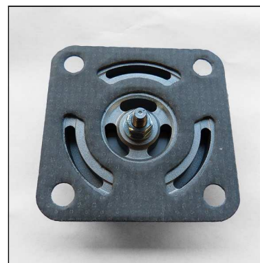
Ensure the correct mounting position of the paper gasket
