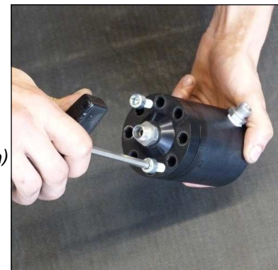
Fig. 2 - Remove the cover
