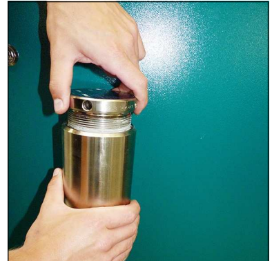
Fig. 1 - Open Filter cover
