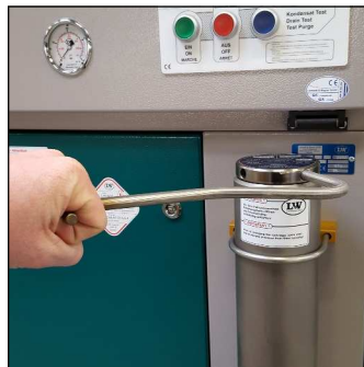
Fig. 2 - Unscrew the filter housing cover.
