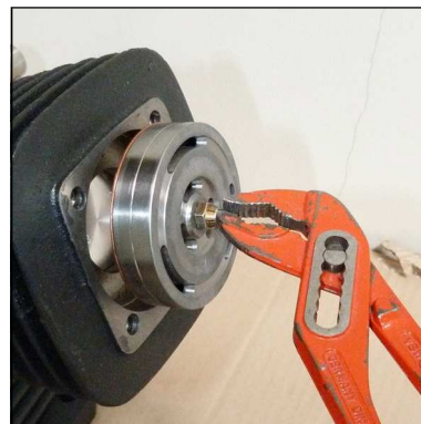
Pull out inlet and outlet valve
