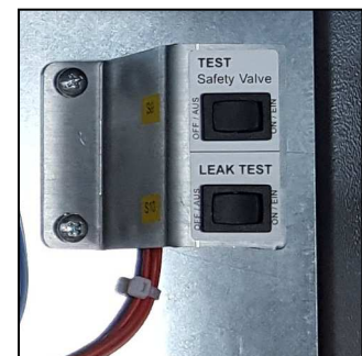
Safety valve test switch (up)
