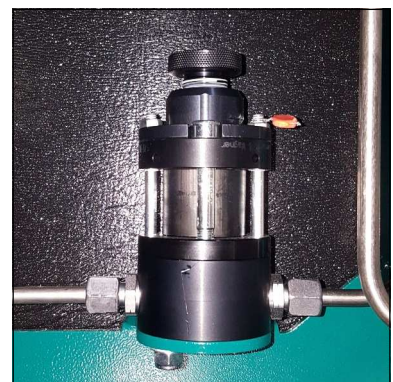
Safety valve 4th stage
