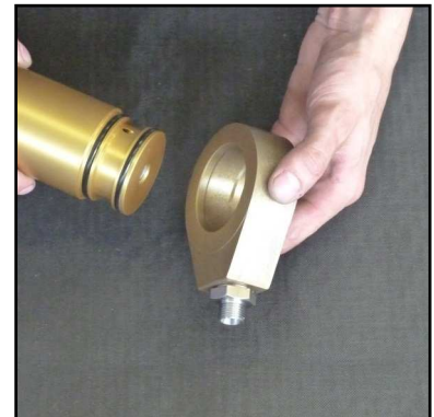
Abb. 6 - Remove the base ring
