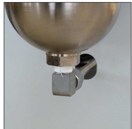
Fig. 2 - Loosen pipes and nuts
