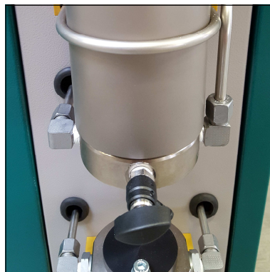
Fig. 3 - Loose pipe connections and nuts
