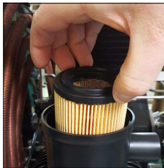
(Fig.2) Remove cover and replace filter cartridge
