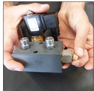
Fig. 3 - Change sinter filter
