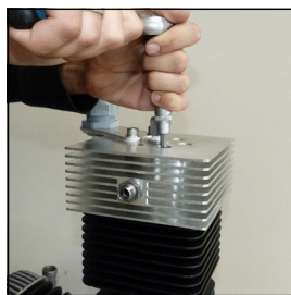
Fig. 1 - Loose valve head screws
