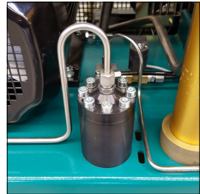
Fig. 1 - Condensate stop valve housing
