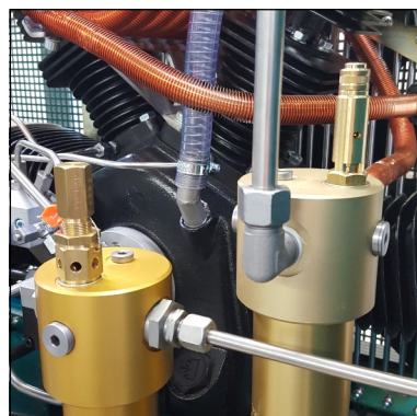
Safety valve 2nd and 3rd stage
