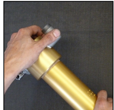
Fig. 1 - Unscrew and remove filter top
