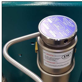
Fig. 2 - Unscrew the filter housing cover.
