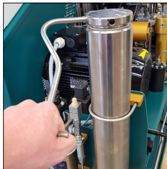
Fig. 2 - Unscrew the filter housing cover.
