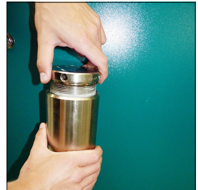
Fig. 1 - Open Filter cover
