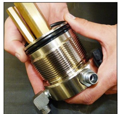
Fig. 4 - Change o-ring and back-up rings
