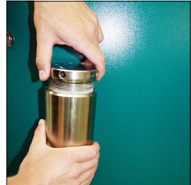
Fig. 1 - Open Filter cover
