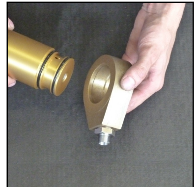
Abb. 6 - Remove the base ring
