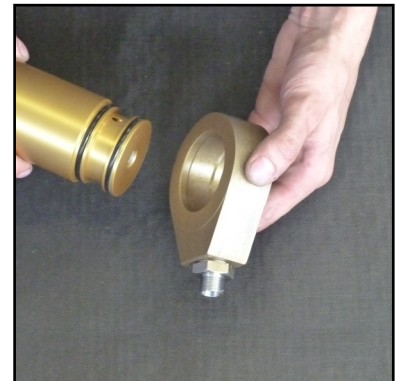
Abb. 6 - Remove the base ring
