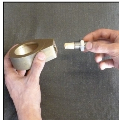
Abb. 8 - Change sinter filter
