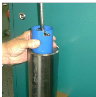
Fig. 4 - Pull the cartridge out of the housing.
