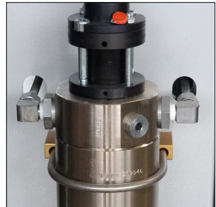
Fig. 1 - Loosen pipes and nuts
