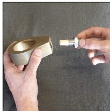
Abb. 8 - Change sinter filter
