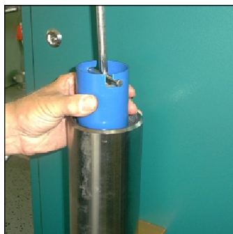
Fig. 4 - Pull the cartridge out of the housing.
