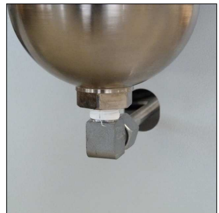
Fig. 2 - Loosen pipes and nuts
