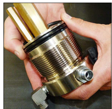
Fig. 4 - Change o-ring and back-up rings
