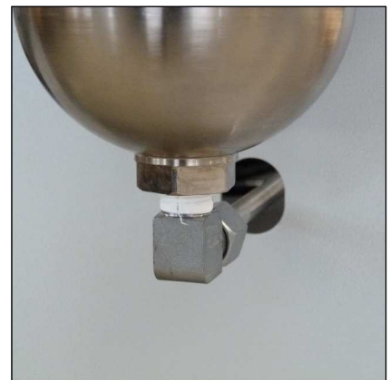
Fig. 2 - Remove HP-pipes and mounting screws
