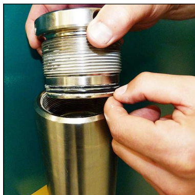
Fig. 2 - Change o-ring and back-up rings
