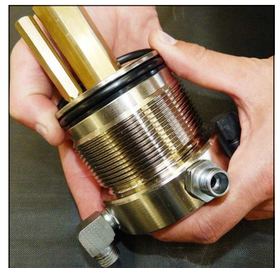
Fig. 4 - Change o-ring and back-up rings
