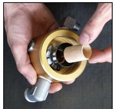
Fig. 3 - Change sinter filter
