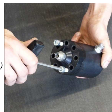
Fig. 2 - Remove the cover
