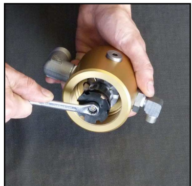
Fig. 2 - Loose nut at the separator top
