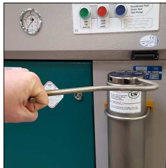
Fig. 2 - Unscrew the filter housing cover.
