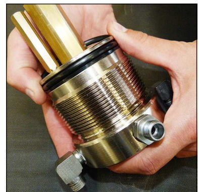
Fig. 4 - Change o-ring and back-up rings
