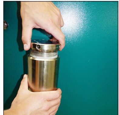
Fig. 1 - Open Filter cover
