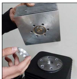
Fig. 2 - Remove lower valve gasket
