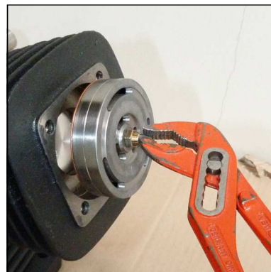
Fig. 2 - Pull out inlet and outlet valve
