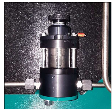
Safety valve 4th stage
