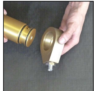
Abb. 6 - Remove the base ring
