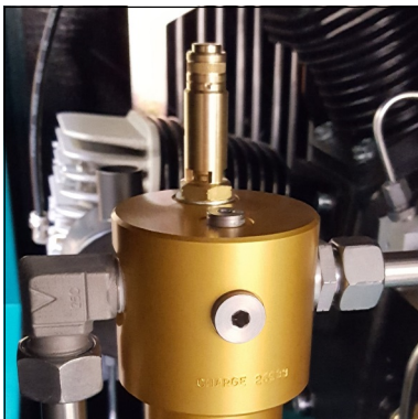
Safety valve 1st stage
