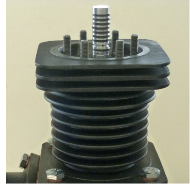
Fig. 1 - take off compression cylinder
