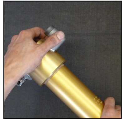
Fig. 1 - Unscrew and remove filter top
