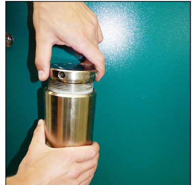
Fig. 1 - Open Filter cover
