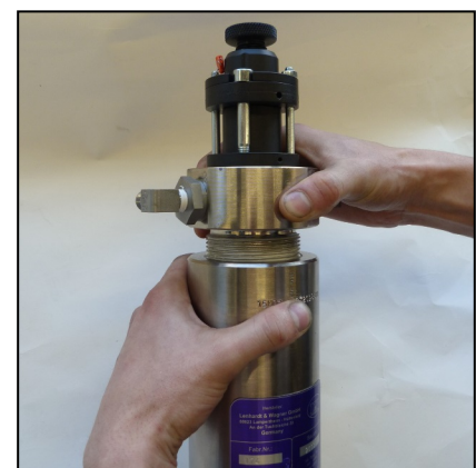
Fig. 3 - Open pre-filter cover
