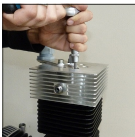
Fig. 1 - Loose valve head screws
