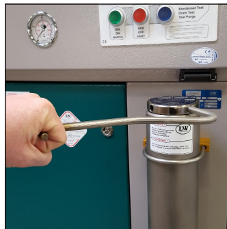
Fig. 2 - Unscrew the filter housing cover.
