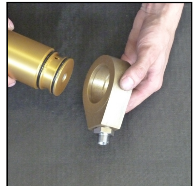
Abb. 6 - Remove the base ring
