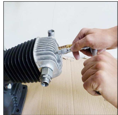
Fig. 1 - Loosen valve head screws
