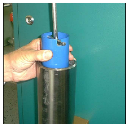
Fig. 3 - Pull the cartridge out of the housing.
