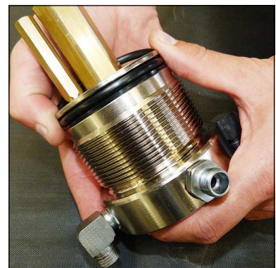
Fig. 4 - Change o-ring and back-up rings
