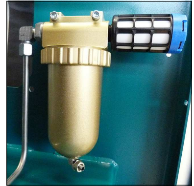
Oil / water separators final stage
