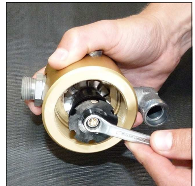
Fig. 2 - Loosen nut at the separator top
