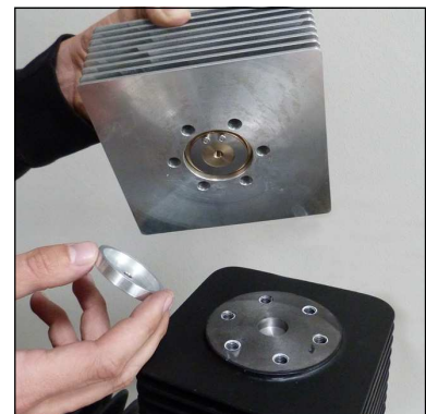
Fig. 2 - Remove lower valve gasket
