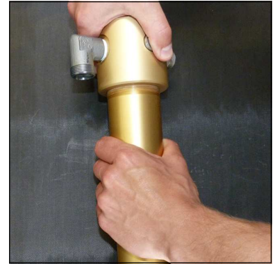
Fig. 1 - Unscrew and remove filter top
