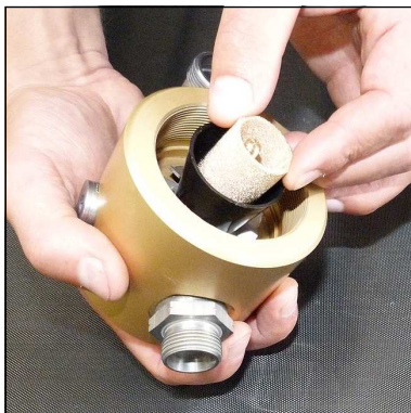
Fig. 3 - Change sinter filter
