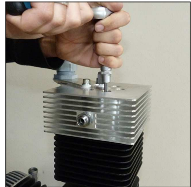
Fig. 1 - Loosen valve head screws
