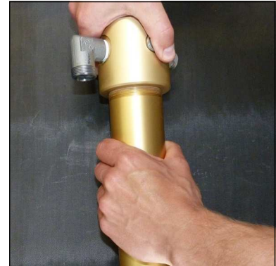
Fig. 1 - Unscrew and remove filter top
