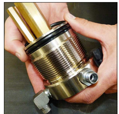
Fig. 4 - Change o-ring and back-up rings
