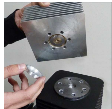
Fig. 2 - Remove lower valve gasket
