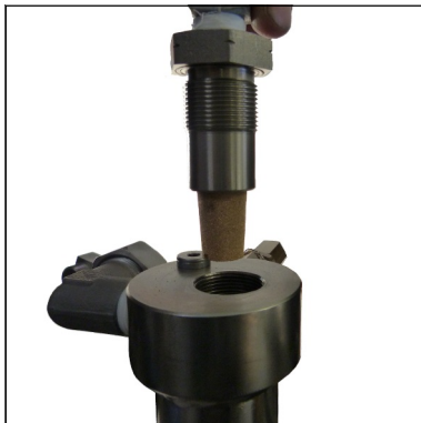
Fig. 2 - Remove sinter filter holder
