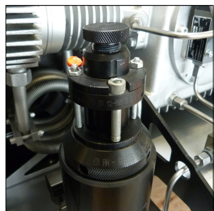
Fig. - Safety valve 3rd stage
