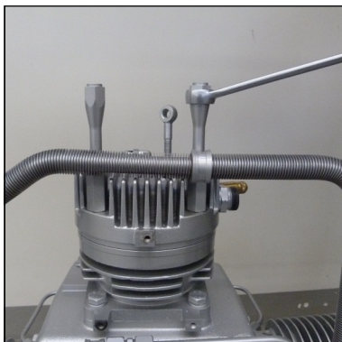
Fig. 5 - Remove cooling pipe bracket
