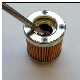
View bypass valve
