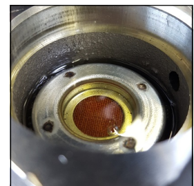
Installation view oil filter
