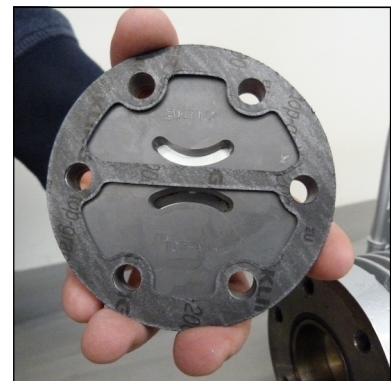
Fig. 2 - Correct mounting position of upper valve gasket
