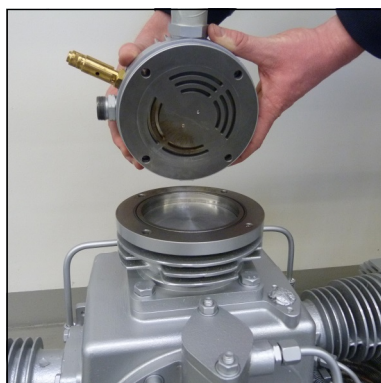
Fig. 3 - Place valve head to cylinder
