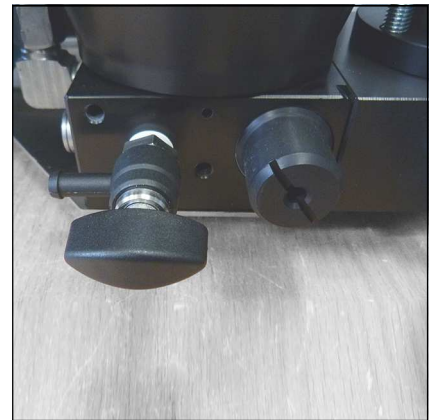
Fig. - Drain valve and pressure maintaining / non return valve
