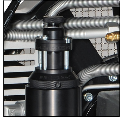
Fig. 1 - Remove/screw in filter cover
