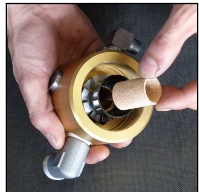
Fig. 3 - Change sinter filter
