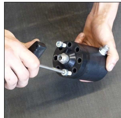
Fig. 2 - Remove the cover
