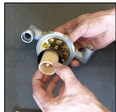
Fig. 3 - Change sinter filter
