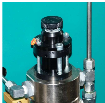
Safety valve 3rd stage
