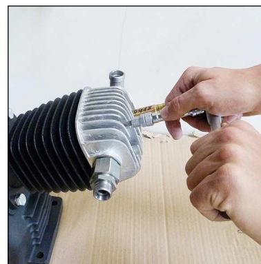
Fig. 1 - Loosen valve head screws
