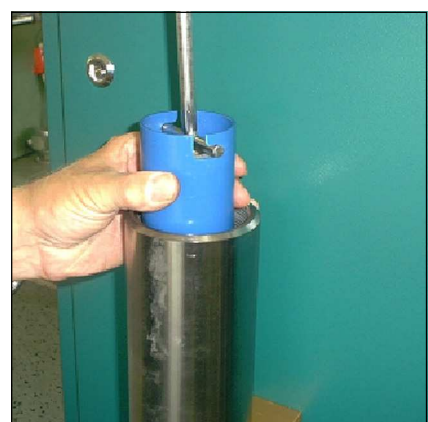
Fig. 3 - Pull the cartridge out of the housing.
