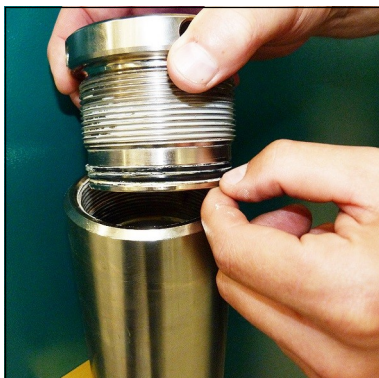
Fig. 2 - Change o-ring and back-up rings
