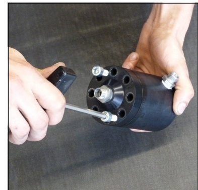
Fig. 2 - Remove the cover
