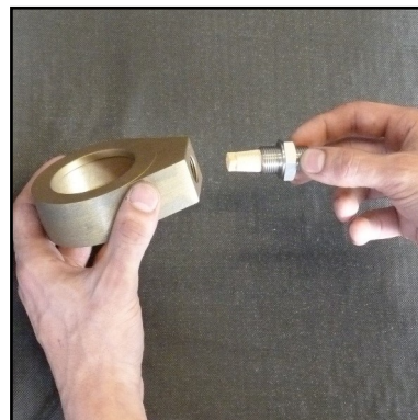
Abb. 8 - Change sinter filter
