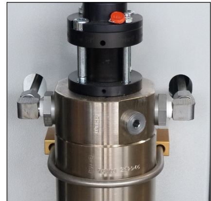
Fig. 1 - Loosen pipe connections and mounting screws
