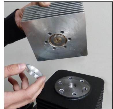
Fig. 2 - Remove lower valve gasket
