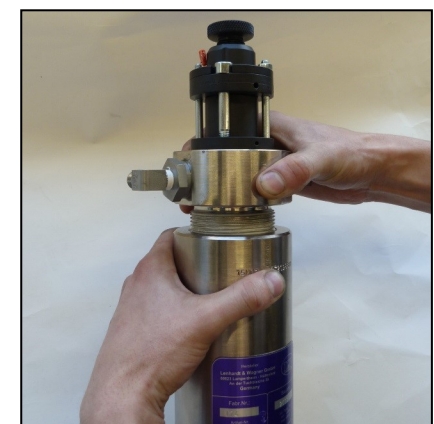
Fig. 3 - Open filter cover
