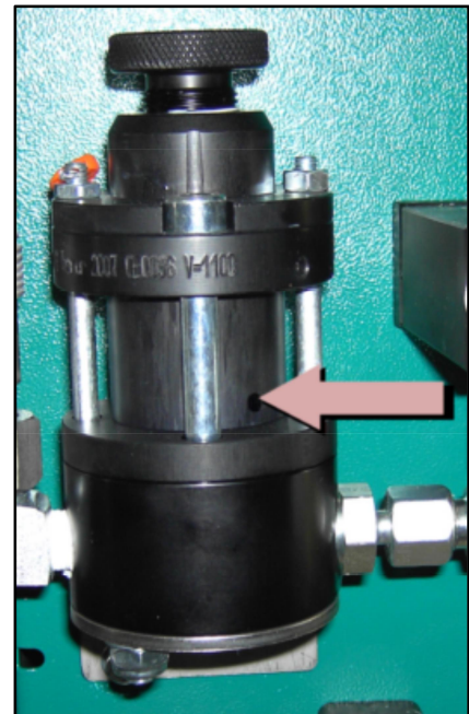
Figure 1: Position for oil refill
