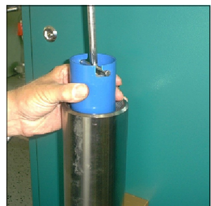
Fig. 3 - Pull the cartridge out of the housing.
