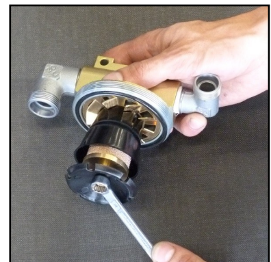
Fig. 2 - Loosen nut at the separator top
