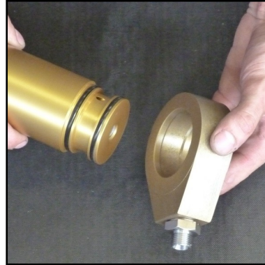
Abb. 5 - Remove the base ring
