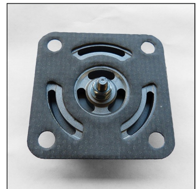
Fig. 4 - Ensure the correct mounting position of the paper gasket
