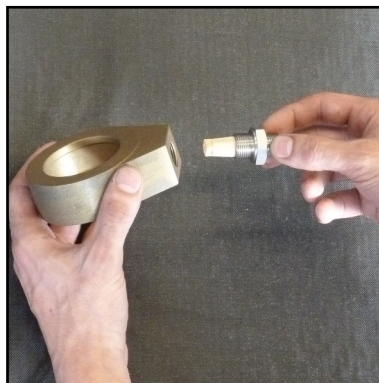
Abb. 7 - Change sinter filter
