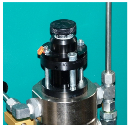
Safety valve 3rd stage
