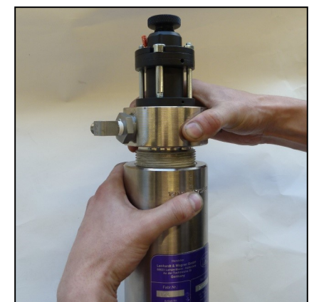
Fig. 3 - Open pre-filter cover
