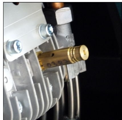
Safety valve 2nd stage
