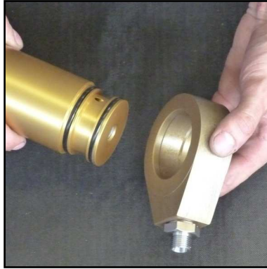
Abb. 5 - Remove the base ring
