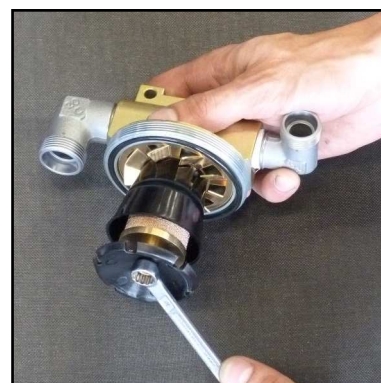
Fig. 2 - Loosen nut at the separator top
