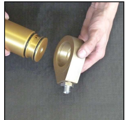
Abb. 6 - Remove the base ring
