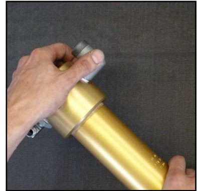
Fig. 1 - Unscrew and remove filter top
