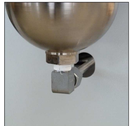
Fig. 2 - Loosen pipe connections and mounting screws
