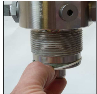
Fig. 1 - Change o-ring and back-up ring
