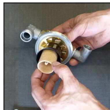
Fig. 3 - Change sinter filter
