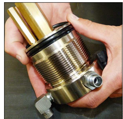
Fig. 4 - Change o-ring and back-up rings
