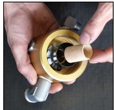
Fig. 3 - Change sinter filter
