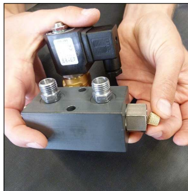
Fig. 3 - Change sinter filter
