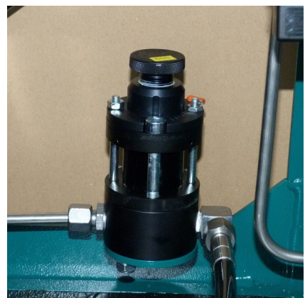
Safety valve 3rd stage
