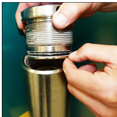
Fig. 2 - Change o-ring and back-up rings
