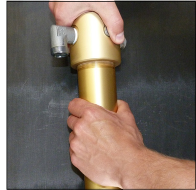
Fig. 1 - Unscrew and remove filter top
