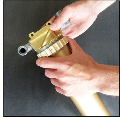
Fig. 1 - Open ring nut and remove separator top
