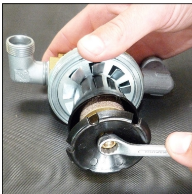
Fig. 2 - Loosen nut at the separator top
