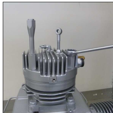
Fig. 6 - Remove special hexagon bolt
