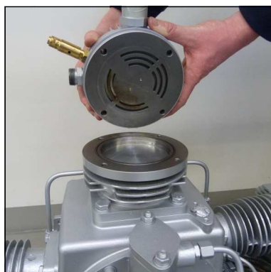
Fig. 3 - Place valve head to cylinder
