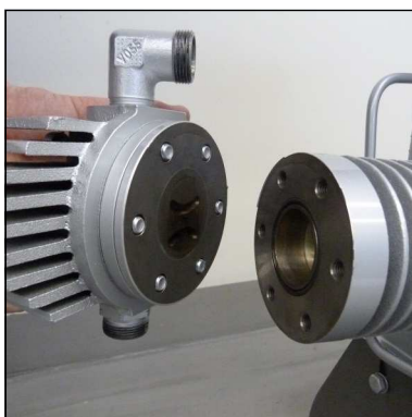
Fig. 3 - Place valve head to cylinder
