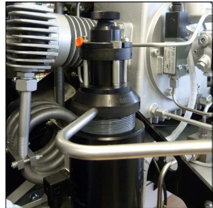
Fig. 1 - Loosen filter housing cover by using the filter tool
