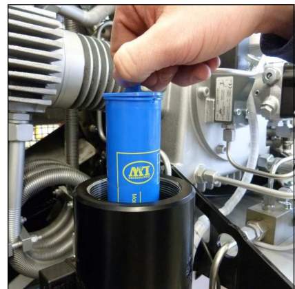
Fig. 2 - Pull out the filter cartridge by the catch and insert a new cartridge
