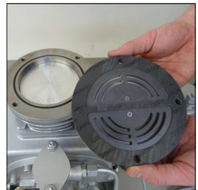
Fig. 2 - Correct mounting position of upper valve gasket
