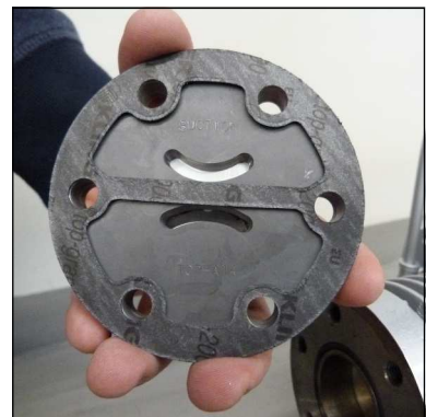
Fig. 2 - Correct mounting position of upper valve gasket
