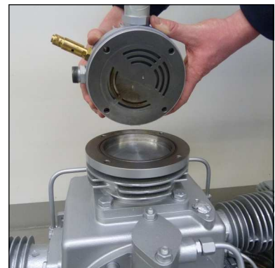
Fig. 7 - Remove valve head
