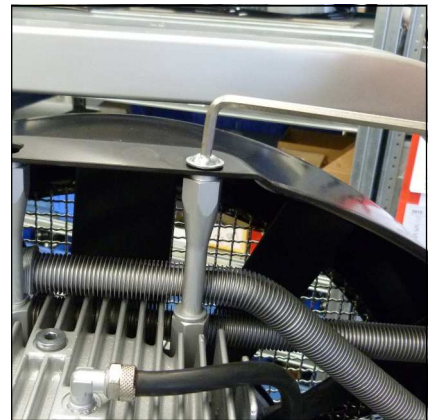
Fig. 1 - Remove top mounting screws
