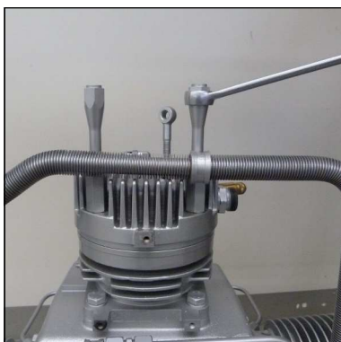
Fig. 4 - Remove cooling pipe bracket
