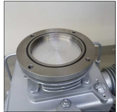
Fig. 1 - Change lower gasket (o-ring)
