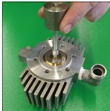
Fig. 4 - Remove inlet and outlet valve
