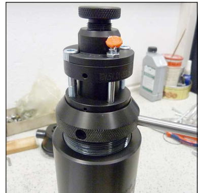
Fig. 1 - Remove/screw in filter cover
