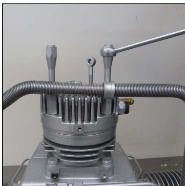
Fig. 5 - Remove cooling pipe bracket
