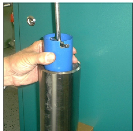
Fig. 3 - Pull the cartridge out of the housing.
