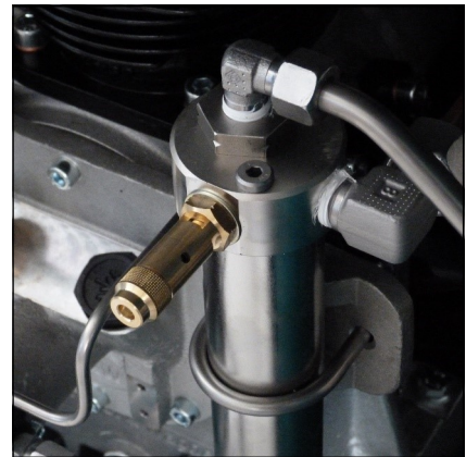
Safety valve 1st stage
