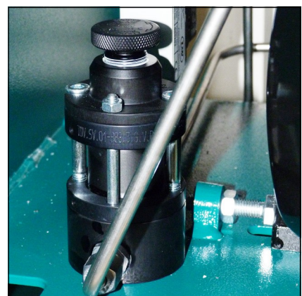
Safety valve 3rd stage
