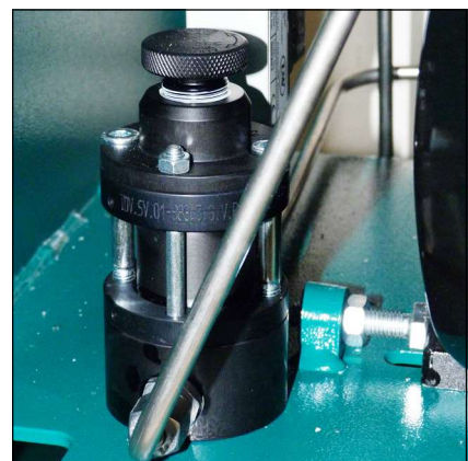
Safety valve 3rd stage
