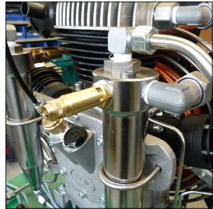
Safety valve 1st stage
