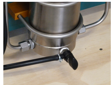
Fig. 2 - Condensate drain valve of the filter housing
