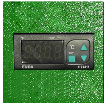
Oil Temperature Monitoring
