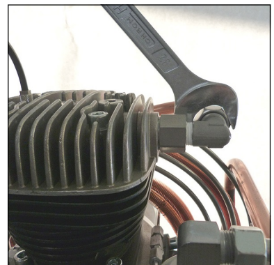
Fig. 6 - Connect pipe connections and tighten
