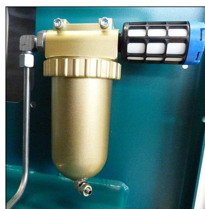
Oil / water separators final stage
