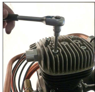
Fig. 5 - Screw valve head screws in
