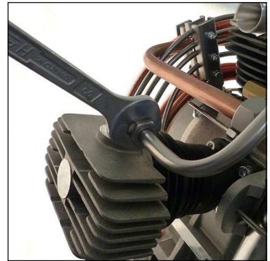
Fig. 1 - Loosen pipe connections
