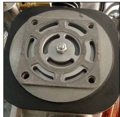
Fig. 4 - Place and align upper valve gasket
