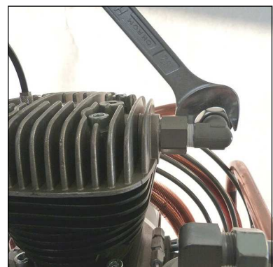
Fig. 6 - Connect pipe connections and tighten
