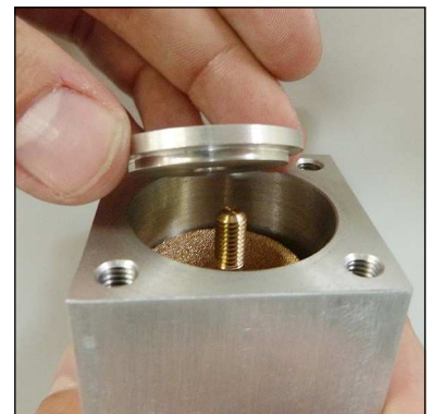
Fig. 5 - Place filter washer and washer
