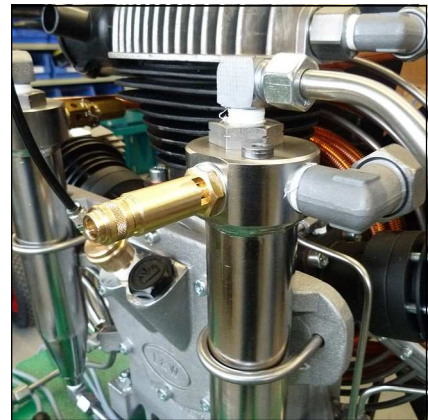
Safety valve 1st stage
