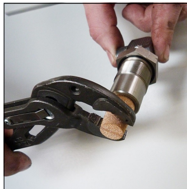
Fig. 3 - Change sinter filter
