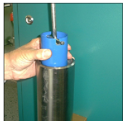
Fig. 3 - Pull the cartridge out of the housing.
