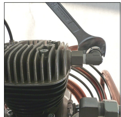
Fig. 6 - Connect pipe connections and tighten
