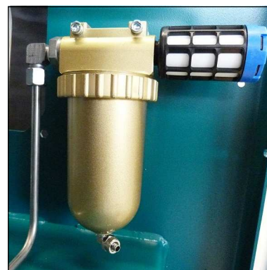
Oil / water separators final stage
