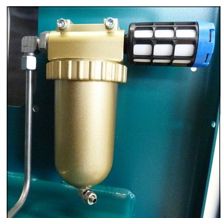
Oil / water separators final stage
