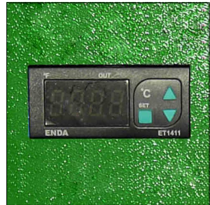
Oil Temperature Monitoring
