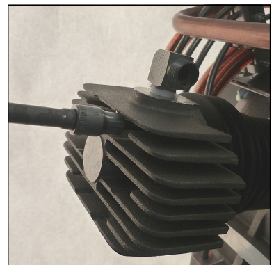
Fig. 2 - Loosen valve head screws
