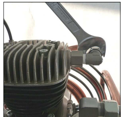
Fig. 6 - Connect pipe connections and tighten
