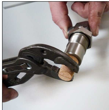
Fig. 3 - Change sinter filter
