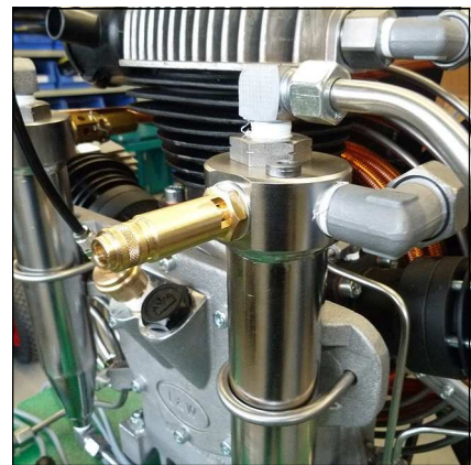
Safety valve 1st stage
