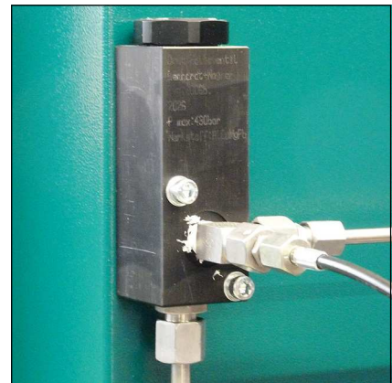
Pressure maintaining/non-return valve
