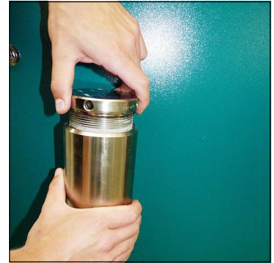
Fig. 1 - Open Filter cover
