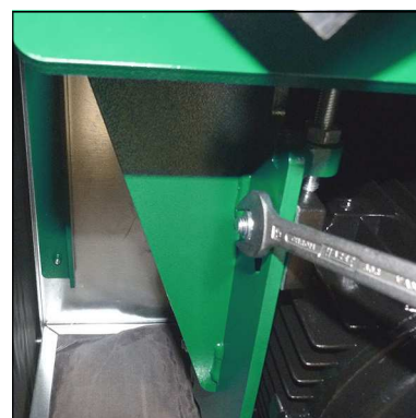
Fig. 1 - Loosen mounting screws
