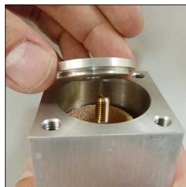
Fig. 5 - Place filter washer and washer
