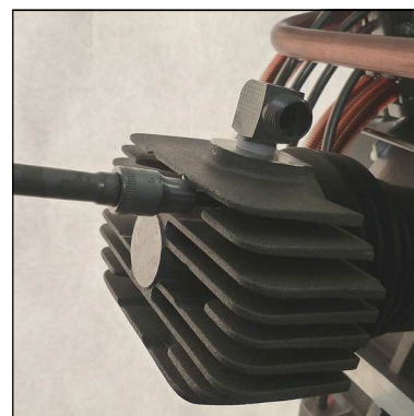
Fig. 2 - Loosen valve head screws
