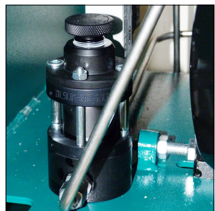
Safety valve 3rd stage
