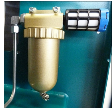
Oil / water separators final stage
