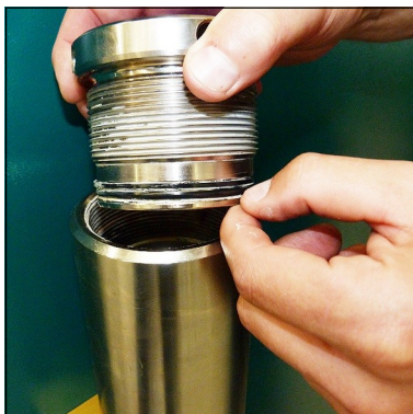
Fig. 2 - Change o-ring and back-up rings
