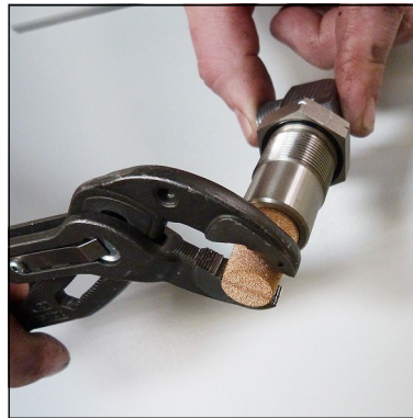
Fig. 3 - Change sinter filter
