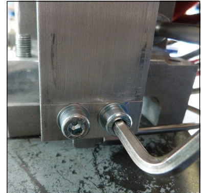
Fig. 1 - Loosen mounting screws
