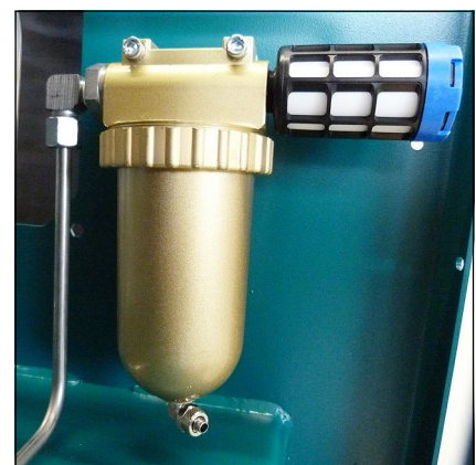
Oil / water separators final stage
