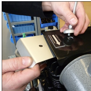
Fig. 2 - Remove protection plate
