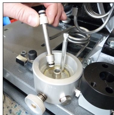
Abb. 5 - Remove duct collar and change o-rings
