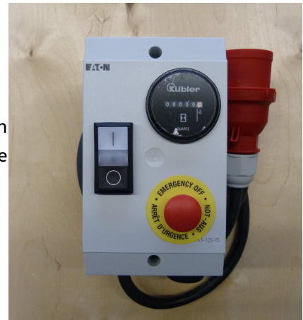
Remote control box c/w hour counter
