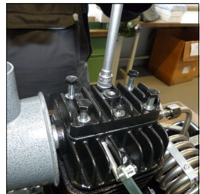
Fig. 4 - Valve head cover screws
