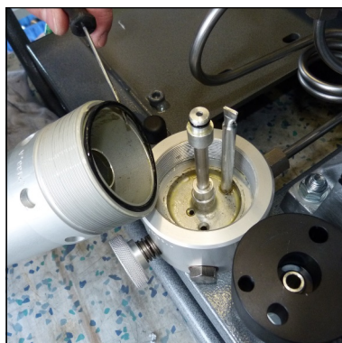
Abb. 4 - Remove lock ring
