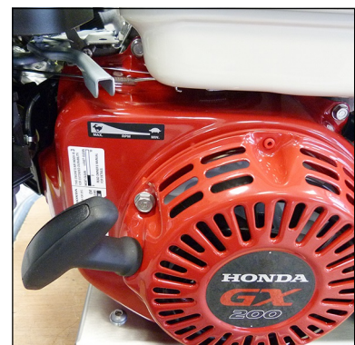
Fig. 2 - Speed control and pull start
