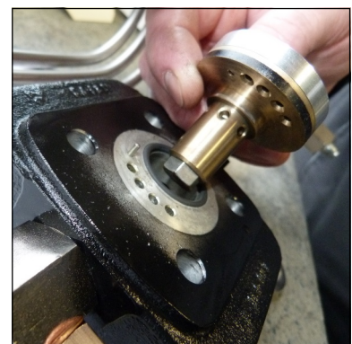
Fig. 5 - Ensure correct valve position (centre pin)
