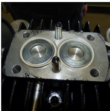
Fig. 5 - Spring plate inside the valve head
