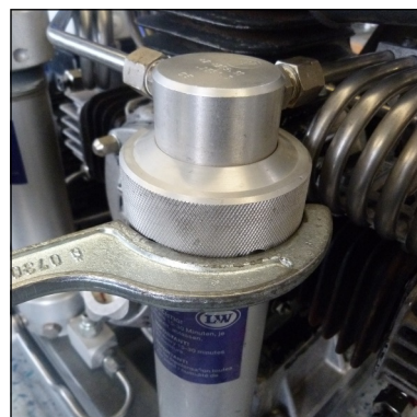
Abb. 5 - Tighten lock ring
