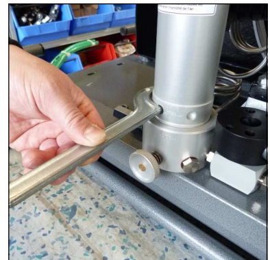
Abb. 3 - Turn off filter housing
