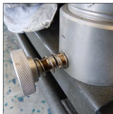
Abb. 6 - O-ring, condensate drain valve
