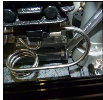
Fig. 2 - Loosen pipe connections of the filter housing
