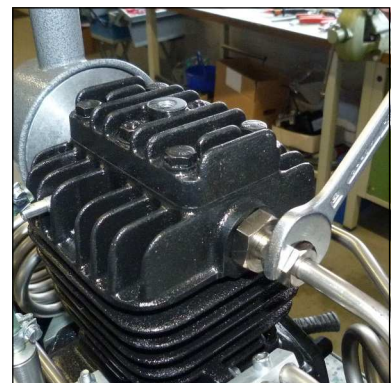
Fig. 7 - Tighten pipe connections
