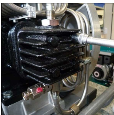
Fig. 2 - Loosen valve head screws
