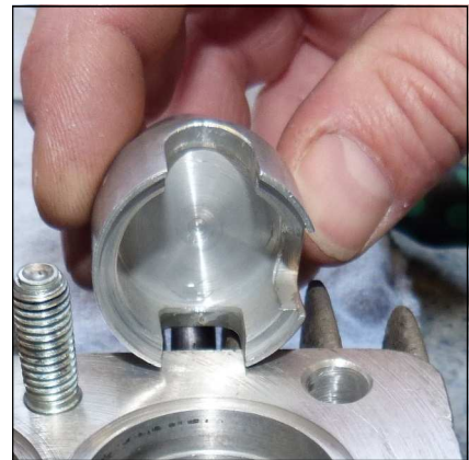
Fig. 1 - Outlet valve holder 1st. stage
