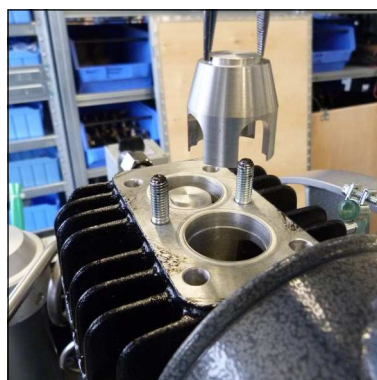
Fig. 6 - Inlet valve bracket
