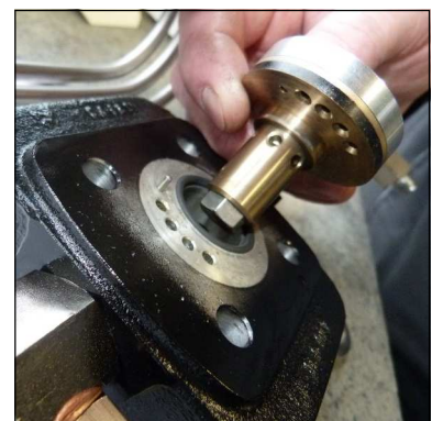
Fig. 5 - Ensure correct valve position (centre pin)
