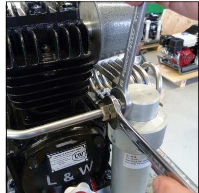
Fig. 1 - Loosen pipe connections of the water separator
