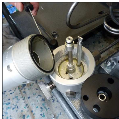
Abb. 4 - Remove lock ring
