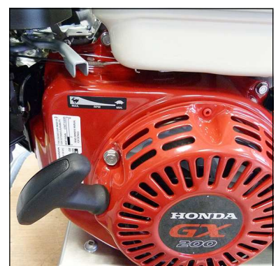
Fig. 2 - Speed control and pull start
