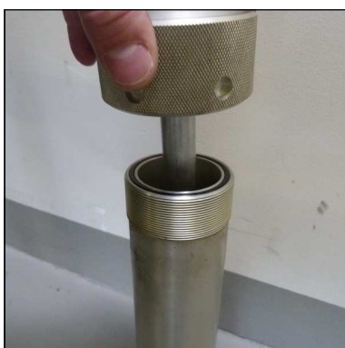
Abb. 4 - Remove lock ring and change o-ring
