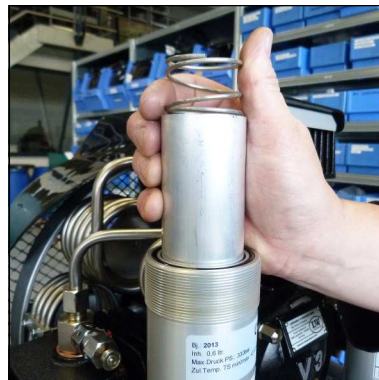
Abb. 2 - Remove filter cartridge
