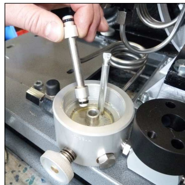
Abb. 5 - Remove duct collar and change o-rings
