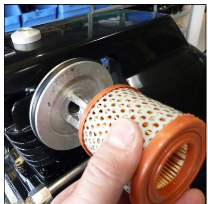
Fig. 3 - Change intake filter
