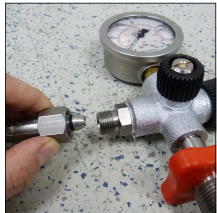
Fig. 2 - O-ring at the filling hose
