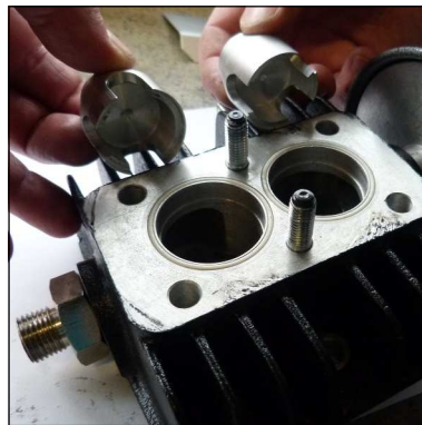
Fig. 3 - Valve bracket positioning
