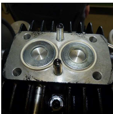
Fig. 5 - Spring plate inside the valve head
