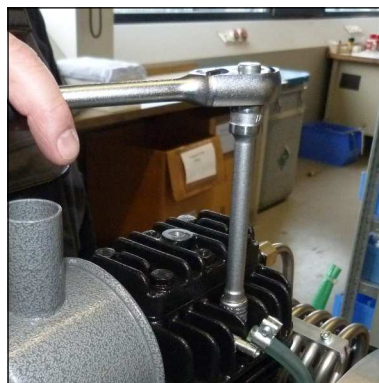
Fig. 6 - Tighten valve head
