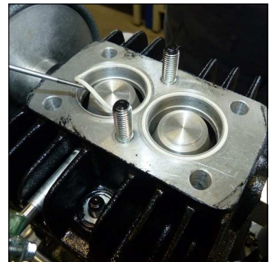
Fig. 4 - Change valve gasket
