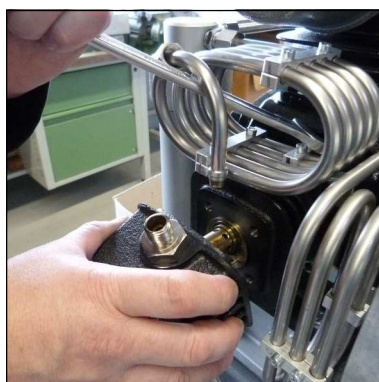
Fig. 3 - Remove valve head
