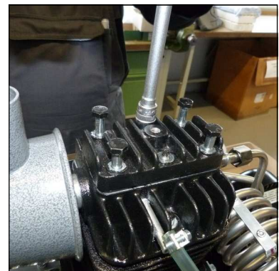
Fig. 4 - Valve head cover screws
