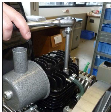
Fig. 3 - Valve head screws
