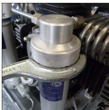
Abb. 5 - Tighten lock ring
