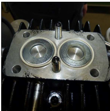
Abb. 5 - Federteller in Ventilkopf
